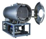
Freeze dryer or freeze dryer - a device designed for canning products by freeze-drying in vacuum.
