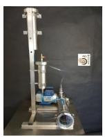
Filtration vacuum station "Mucus filter" for filtering shellfish mucus and other biological fluids under pressure, filtration range 0.2-100 microns. Washable filter elements.
