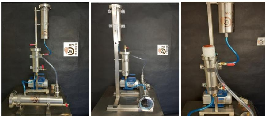
Filtration vacuum station "Mucus filter" for filtering shellfish mucus and other biological fluids under pressure, filtration range 0.2-100 microns.
