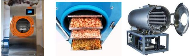
Freeze dryer or freeze dryer - a device designed for canning products by freeze-drying in vacuum.
