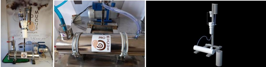
Microfiltration station "Mucus Filter" for filtering mucus from mollusks and other biological fluids under pressure, filtration range 0.2-100 microns. With the possibility of flushing the filter elements.
