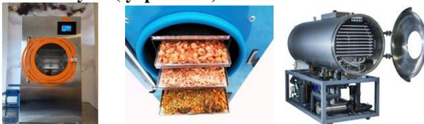
Freeze dryer or freeze dryer - a device designed for canning products by freeze-drying in vacuum.
